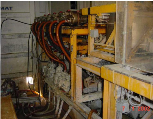
Pump container for grouting the injection pipes
