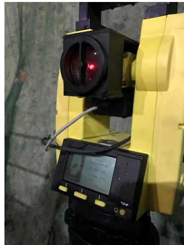
optical total station is watching inside the drill pipe the pilot head
